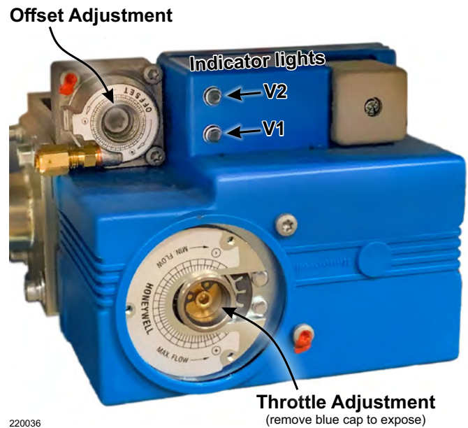
Figure 67 Throttle and offset regulating screws
