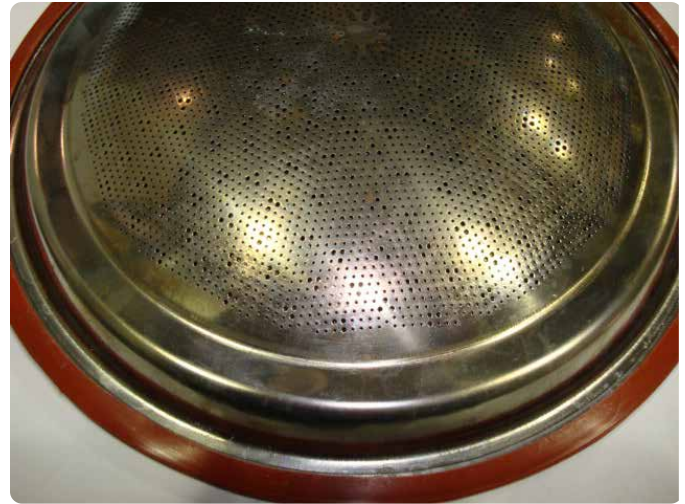
Figure 148 Inspecting exterior and cleaning the burner
