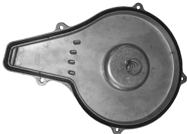
Figure 145 Heat exchanger cover plate removed
