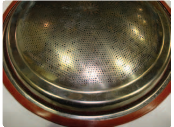
Figure 148 Inspecting exterior and cleaning the burner
