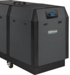
SlimFit 550–2000 MBH models offer the perfect solution for older heating systems in need of an upgrade with a low, horizontal profile. The cast heat exchanger sectional design appeals to cast iron boiler loyalists that need condensing high-efficiency performance and large forgiving waterways to accommodate older boiler plant water systems.
