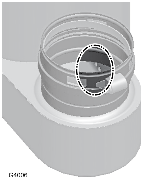
Figure 83 Recuperator flue way drain holes
