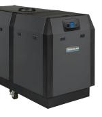
SlimFit 550-2000 MBH models offer the perfect solution for older heating systems in need of an upgrade with a low, horizontal profile. The cast heat exchanger sectional design appeals to cast iron boiler loyalists that need condensing high-efficiency performance and large forgiving waterways to accommodate older boiler plant water systems.
