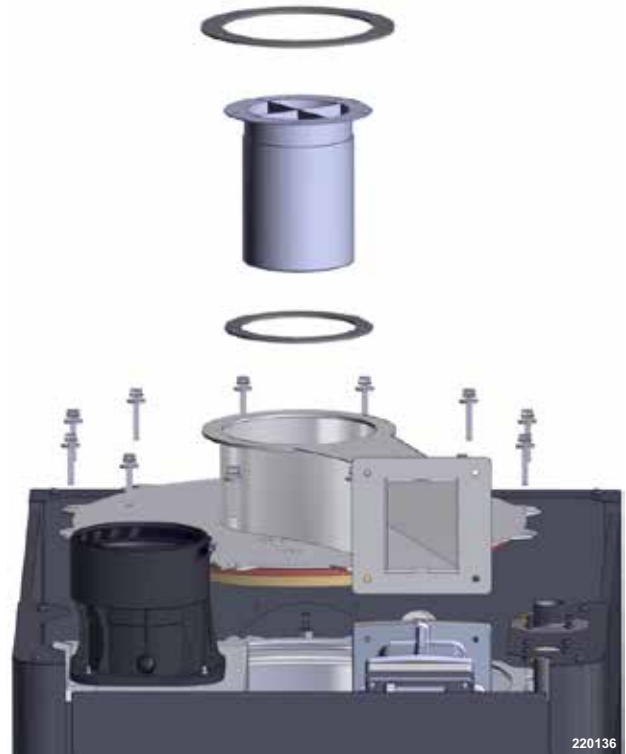
Figure 58 Cover plate and gasket installation
