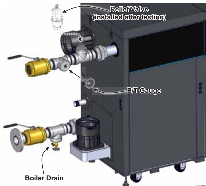
Figure 7 Hydrostatic test piping connections - flanges, valves, and gaskets provided by installer
