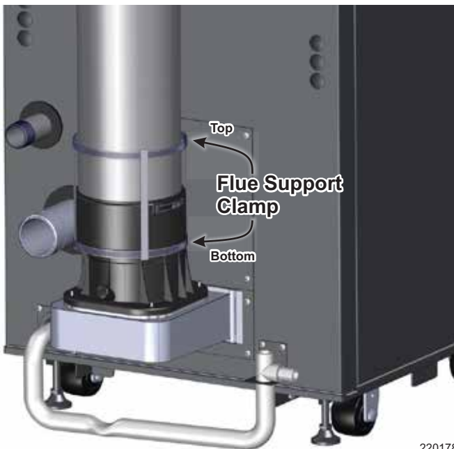
Figure 21 Flue support clamp, installed
